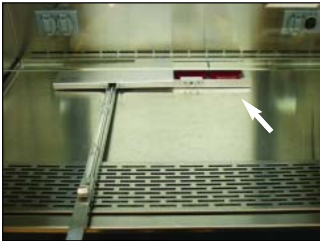
Image 2 _Two of 3 inoculated Petri dishes being exposed at the center rear of the BSC.
