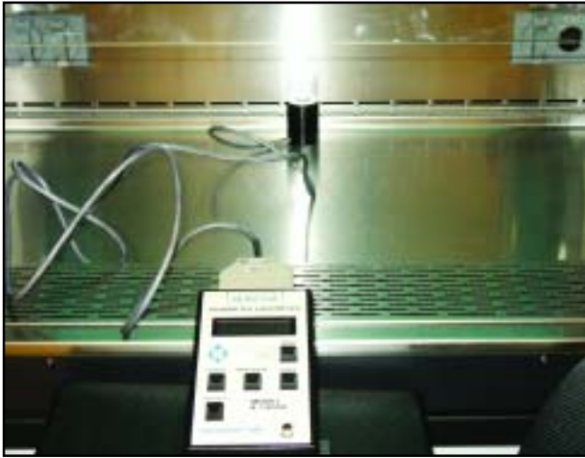
Image 1 _The IL1400A meter, with the UVC detector in position at the center rear of the authors' BSC.
