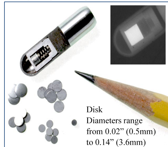
Figure 8.4 (Ir-192 radiography disk sources, with a pencil for size reference)
