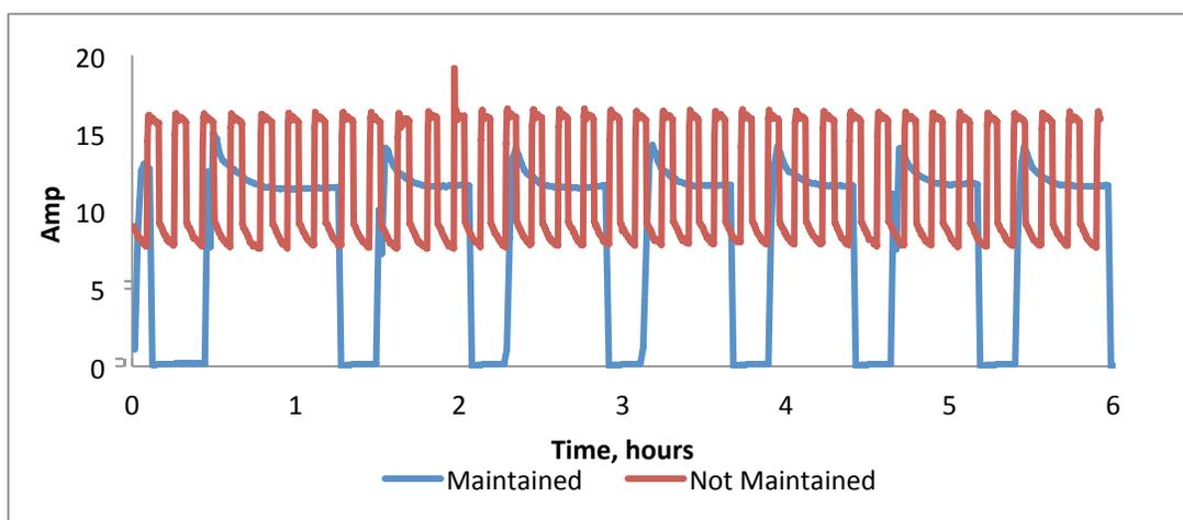
Figure 5 The influence of dust accumulation on ULT freezer filters and condenser fins on amperage for ULT freezers at a set point of  $-80^{\circ}\text{C}$  operating in ambient temperatures from  $23^{\circ}\text{C}$  to  $25^{\circ}\text{C}$  (Gumapas and Simons, 2013)
