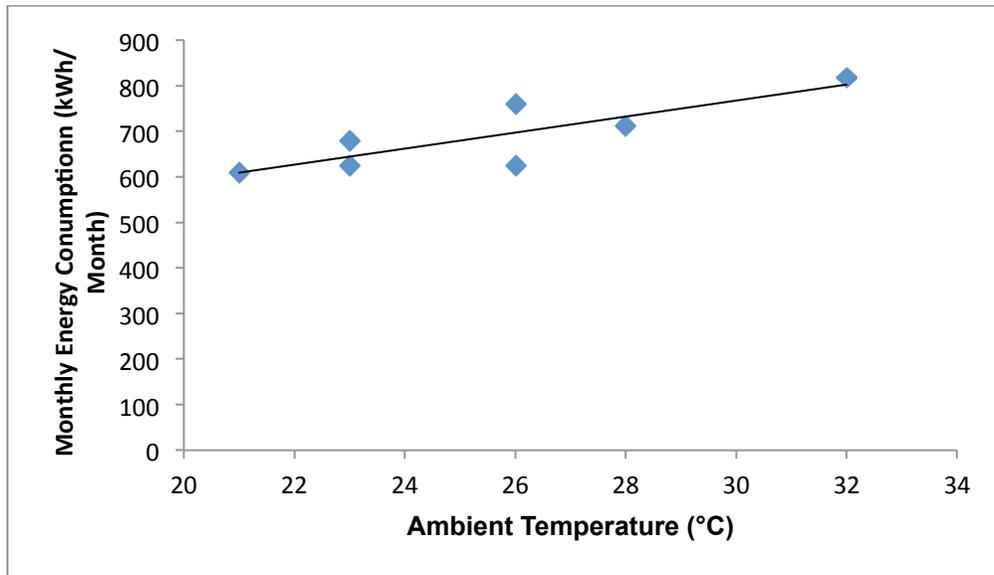
Figure 12 Energy Consumption versus Ambient Temperature for 17.3 ft<sup>3</sup> at set point -80°C for maintained ULT freezers (Gumapas and Simons, 2013)
