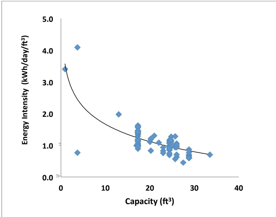
Figure 2 Energy intensity of existing ULT freezers. Freezers smaller than 15 ft<sup>3</sup> use up to three times more energy per volume than 20-25 ft<sup>3</sup> ULT freezers. (Gumapas and Simons, 2013)
